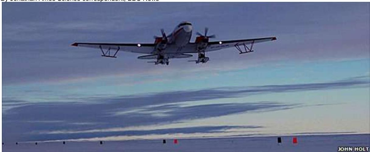
The DC-3 departs from Casey Station. The ice-penetrating radar antennas can be seen under each wing
