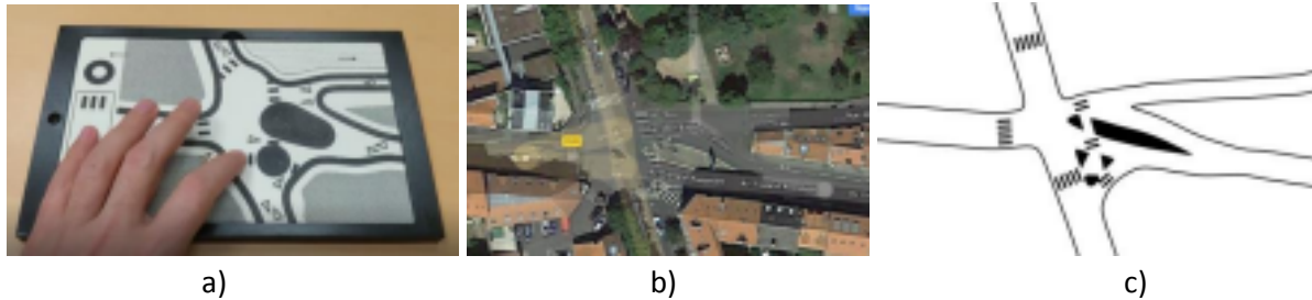
Figure 1. Mapping an intersection and possible interactions. a) a street intersection (Source: Google Maps); b) map produced by the pipeline; c) a first experiment of an interactive map using a swell paper tactile cover on top of a tablet, with audio descriptions for streets and pedestrian crossings.
